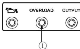
The overload indicator light ① comes on when an overload of a connected electrical device is detected, the inverter control unit overheats, or the AC output voltage rises. Then, the AC protector will trip, stopping power generation in order to protect the generator and any connected electric devices. The AC pilot light (Green) will go off and the overload indicator light (Red) will stay on, but the engine will not stop running.
