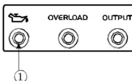
When the oil level falls below the lower level, the oil warning light ① comes on and then the engine stops automatically. Unless you refill with oil, the engine will not start again.
